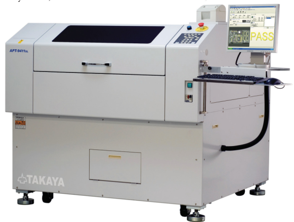
Texmac demonstrated the Takaya APT-9411SL, which the company said is designed to test the large, technically advanced PCBs employed in US telecommunications, high-end-computing, and defense-electronics industries. Base price is less than $300,000. Courtesy of Takaya.
